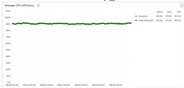
Figure: The CMS HammerCloud jobs CPU efficiency for a \approx 10 km CE-SE distance.
