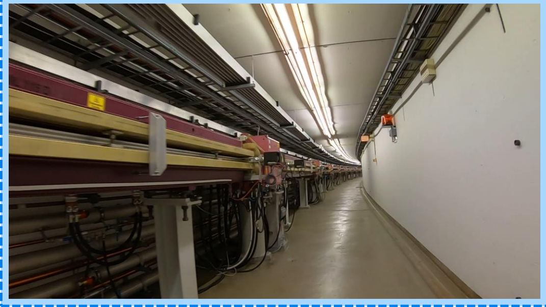
Injection, FoDo cell structure, acceleration cavities
