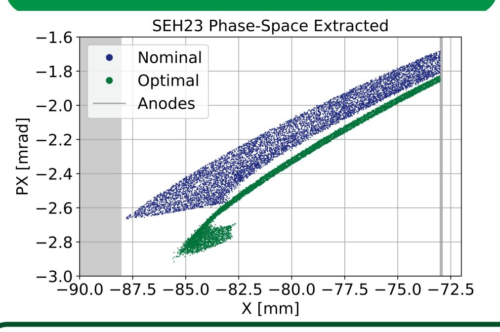
Slow extraction provides continuous beam over seconds: Used in PS East Area for electronic irradiation tests. Applying technique from SLAWG to reduce septum QSE29 losses during extraction by 'folding' separatrices. • Increasing number of particles in **SEH23 field**-region.
