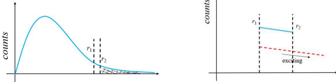
Figure 2: Radial beam distribution with two region's boundaries.
