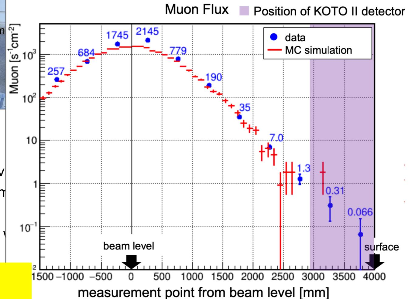
Muon flux is as expected. → 2.1 MHz at KOTO II
