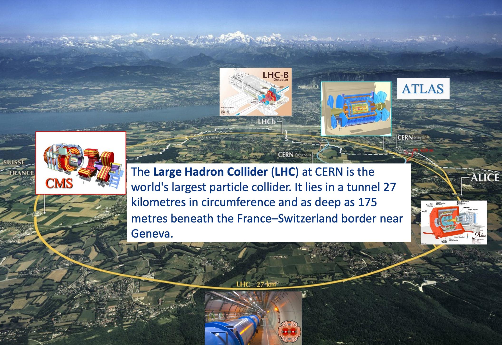
The **Large Hadron Collider (LHC)** at CERN is the world's largest particle collider. It lies in a tunnel 27 kilometres in circumference and as deep as 175 metres beneath the France–Switzerland border near Geneva.
