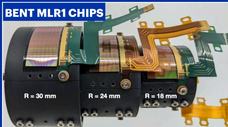
**No performance degradation observed when bending**
