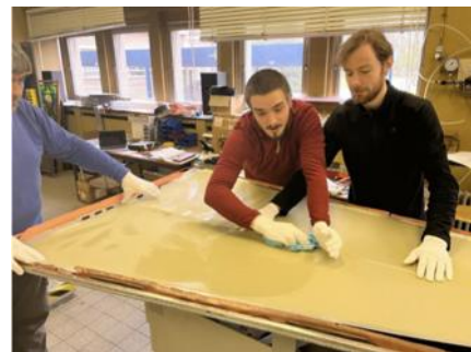
Leak test (drop < 0.4 mbar/10 min)
