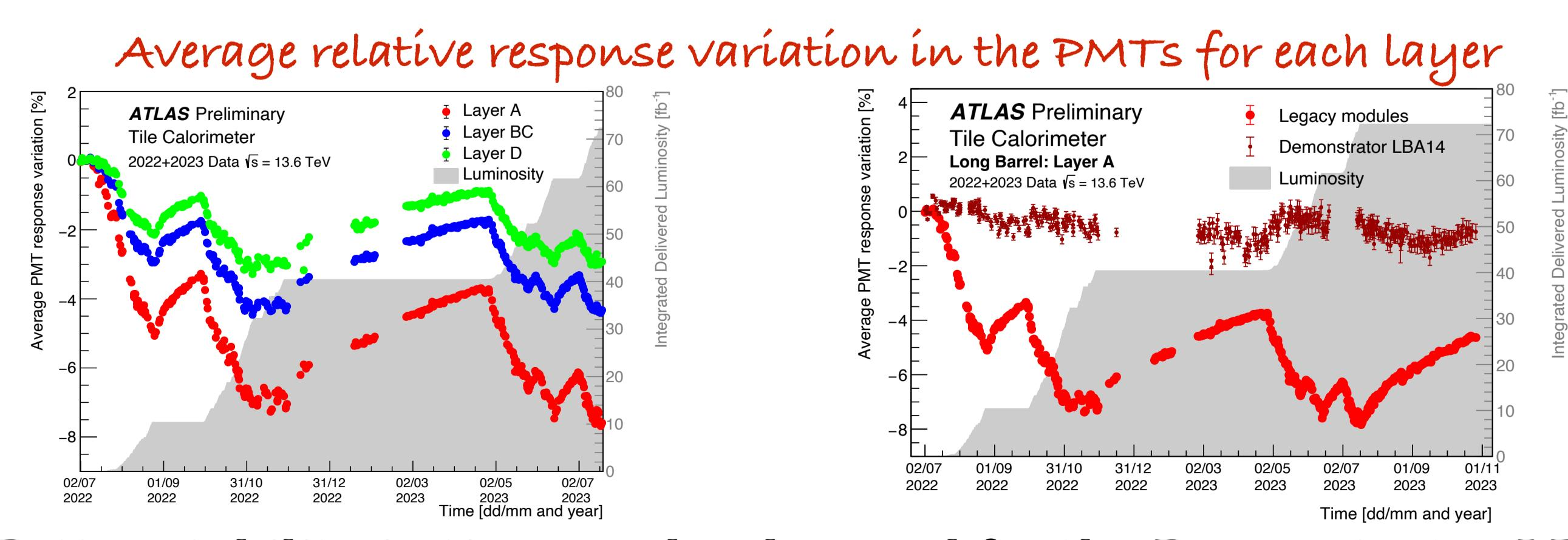
⇒ Better stability in time can be observed for the Demonstrator LBA14 (newer PMT model [Hamamatsu R11187-SEL])
