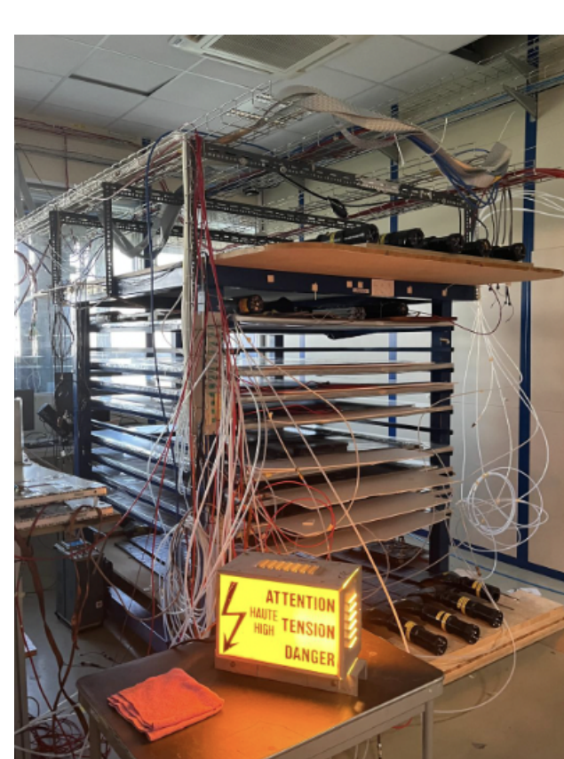
Figure 4: Cosmic test stand for gaps validation
