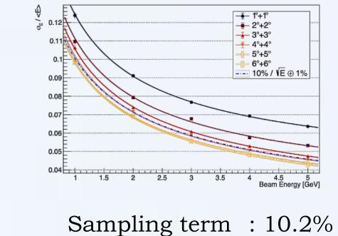
Lead + polystyrene Energy resolution (DESY & SPS, R14755U-100)
