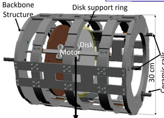
Successful test of JPE piezo motor at 5 K and 5.3 T (ALP magnet @DESY)
