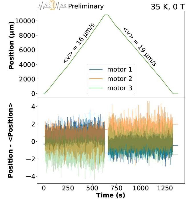
Validated piezo motors and mechanics for open booster
