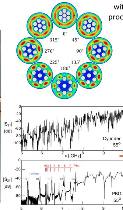
Tunable symmetric lattice resonator with PBG for TE mode suppression; proof of concept for ALPHA 10-20 GHz resonator
