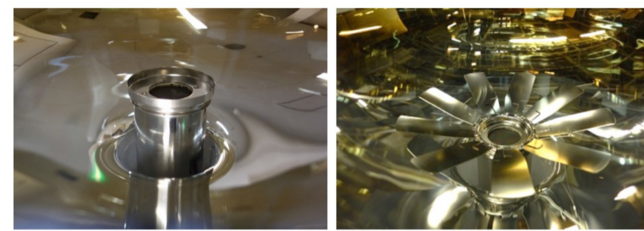
• Photograph of the electrode for the LPMT (left) and lotus-like LPMT (right)
