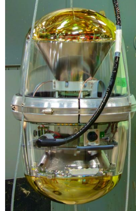
IceCube Upgrade D-Egg (2x8" PMTs)
