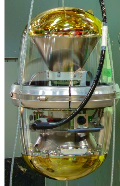
IceCube Upgrade D-Egg (2x8" PMTs)
