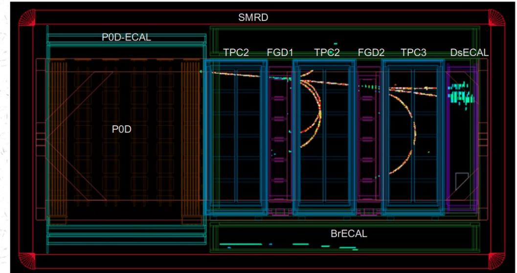
Detector installed inside the **UA1/NOMAD magnet (0.2 T)**
