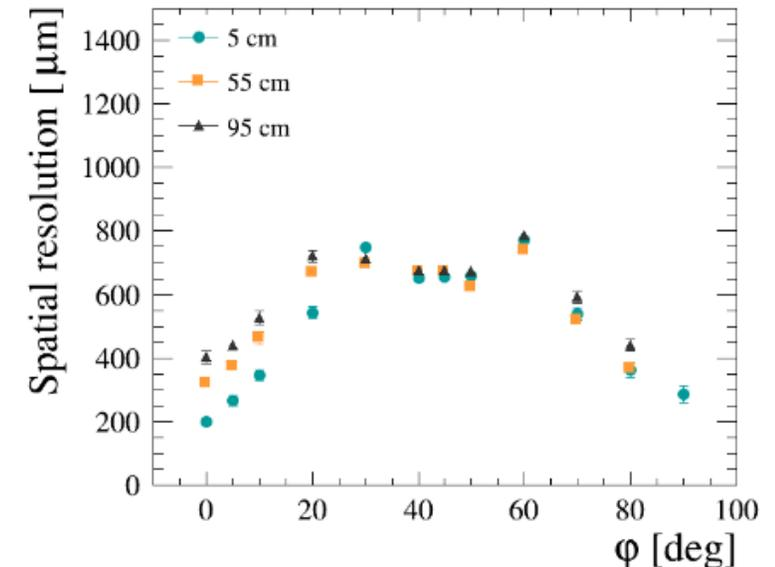
➔ Spatial resolution better than 800  $\mu\text{m}$  and dE/dx resolution better than 10% obtained for all the incident angles and drift distances of interest.
