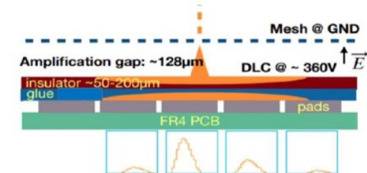
resistive Micromegas (used in HATPC)
