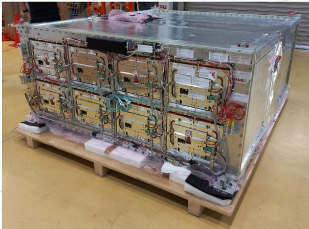
➔ New field cage design with thin walls to minimize dead space and maximize tracking volume. (Total width  $\approx 4$  cm /  $2\% X_0$ )
