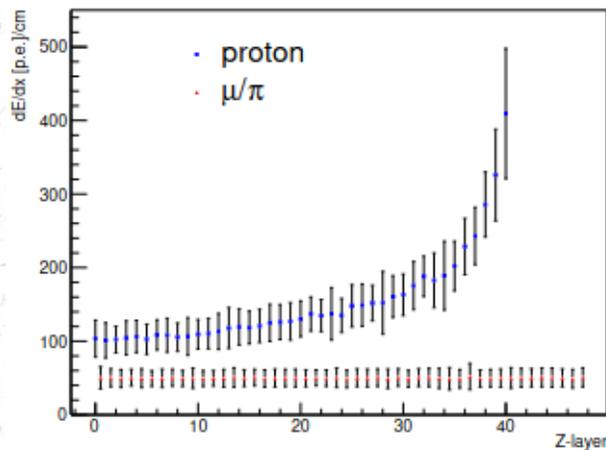
dE/dx resolution v/s no. of cube layers traversed
