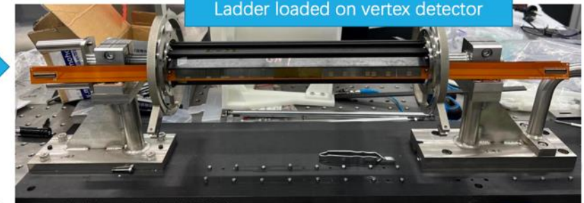
Ladder loaded on vertex detector
