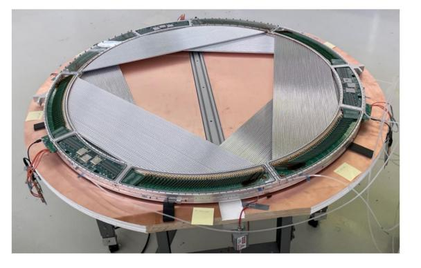
The straw-tube tracker is located in a 1T uniform magnetic field. It is approximately 3 m long and consists of 18 tracking stations with 1152 straws per station. The straws are filled with 80%: 20% Ar: CO<sub>2</sub> mixture.
