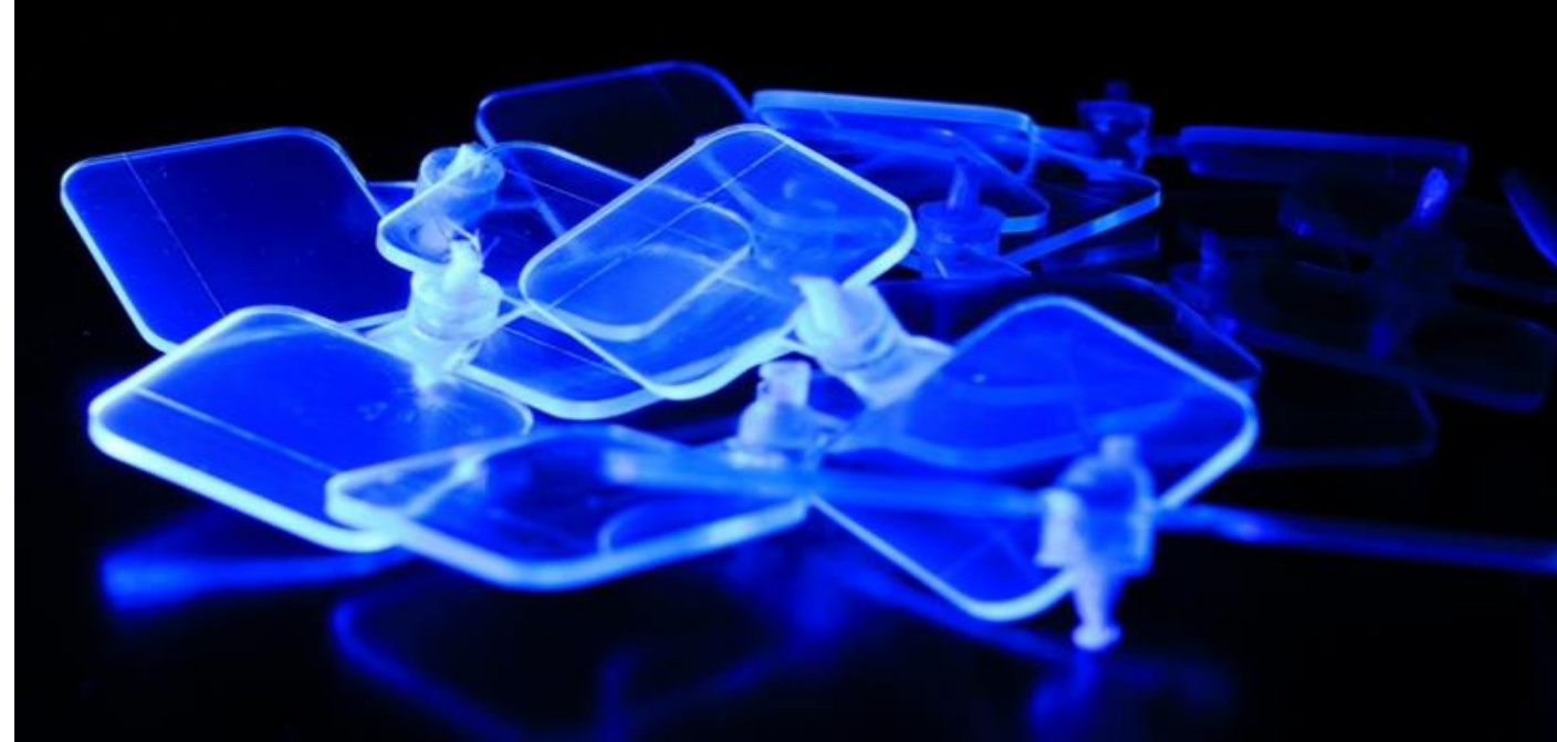
Light response of PEN samples to UV source Picture by Agostinho Gomes
