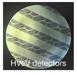
Top right: KID made of 50 nm AlMn on Si (credit: Zoe Smith) Bottom right: HVeV detector made of 600 nm Al/40nm W on Si (credit: Aviv Simchony)
