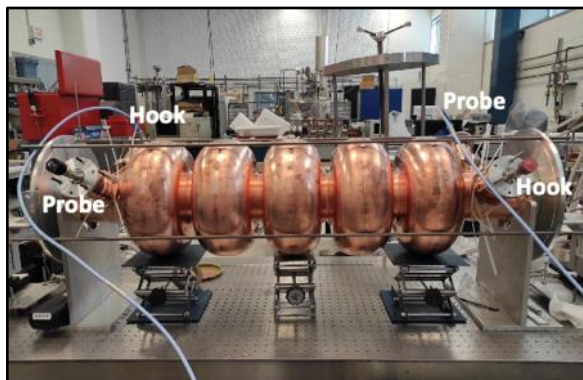
3D-printed prototype (Epoxy Accura 48) copper-coated @CERN
