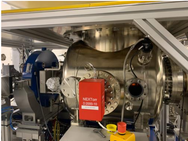
A DC Gun, Cornell design (400 pC, 50 MHz demonstrated), fully equipped (all pumps) in load-lock version
