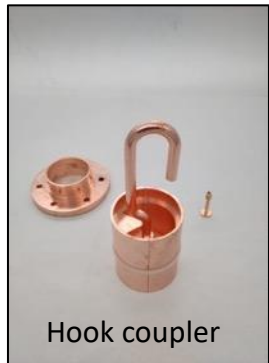
3D-printed prototype (Epoxy Accura 48) copper-coated @CERN
