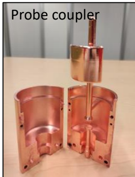
3D-printed prototype (Epoxy Accura 48) copper-coated @CERN
