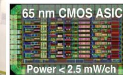
65 nm CMOS ASIC Power < 2.5 mW/ch
