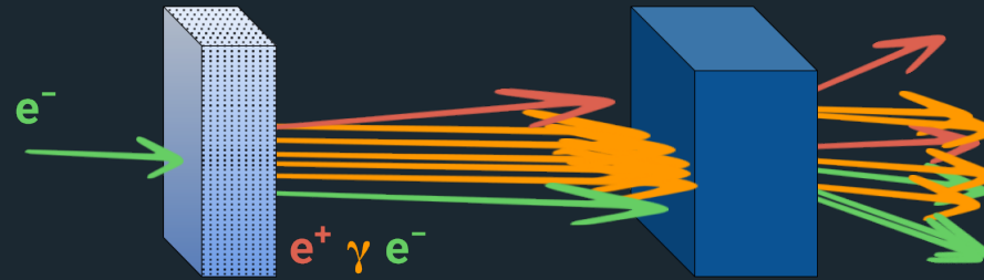
"Thin" crystal ( < X_0 ) photon radiator Amorphous target-converter
