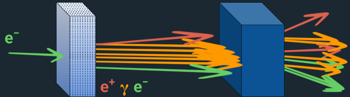
"Thin" oriented crystalline target ( < X_0 ) photon radiator
