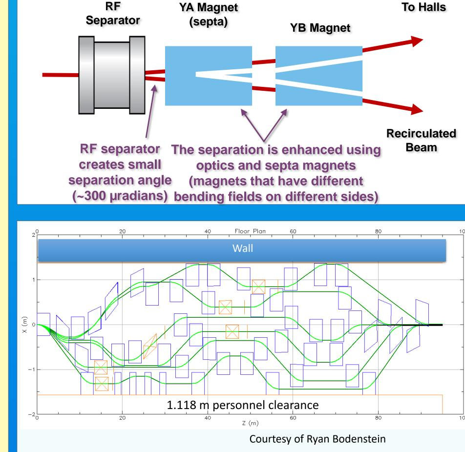
Horizontal Extraction at 750 MHz with three beams left and one beam right
