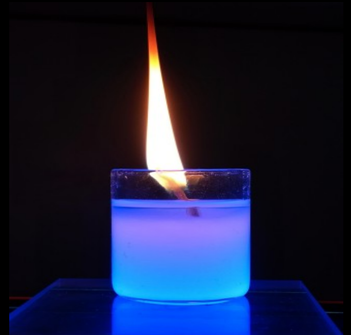
Candle built from NoWaSH (opaque wax-based scintillator)
