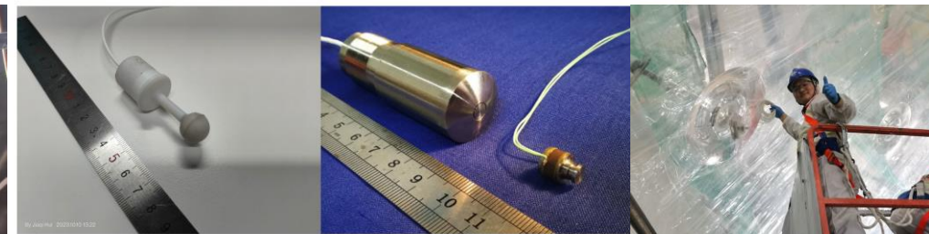
USS emitter (left), receiver (middle) and installation (right)
