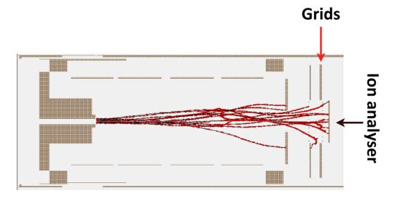
Thermalization chamber simulation: ions passing through the capillary can reach the analyser
