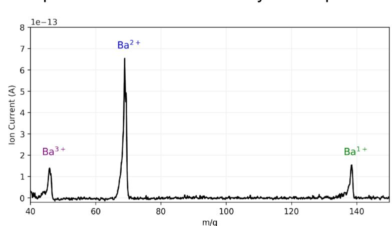
Mass to-charge spectrum at the velocity filter, with the dominant ions, Ba1+, Ba2+ and Ba3+ at 138, 69 and 46, respectively.
