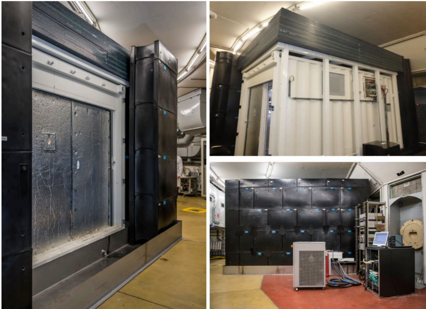
The SoLid container at BR2 prior to completion of water wall
