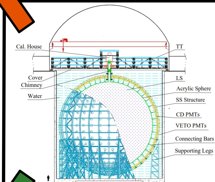
Jiangmen Underground Neutrino Observatory (JUNO) is a 20 kton, radiopure, multi-purpose liquidscintillator detector located in South China.
