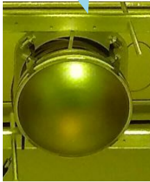
Left & right: uncoated and coated PMTs installed in PDS Box
