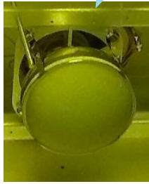
Left & right: uncoated and coated PMTs installed in PDS Box
