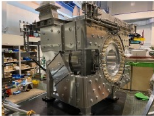
New Horn1 & 2 w/ upgraded cooling capability
