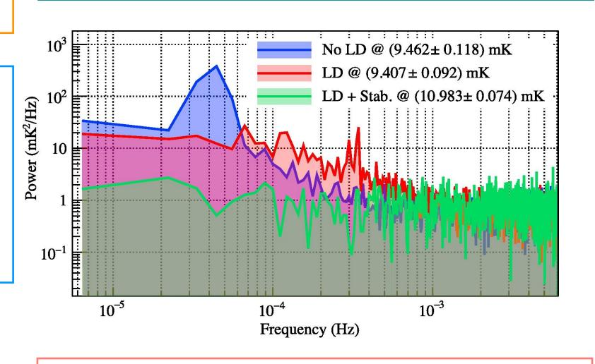
Denoising of the continuous data using ancillary diagnostic devices
