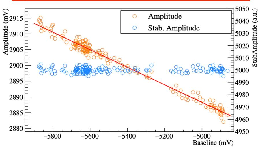
Filtered signal amplitude is corrected against T drifts with fixed E pulses
