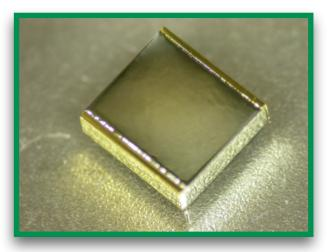
Operating at a temperature of  $\sim 10$  mK: I MeV energy release causes  $\Delta T \sim 100$  µK. We use a Si heater to inject stable voltage pulses and do thermal gain stabilization
