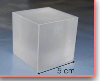
Ge-NTD thermistor  $R \propto e^{\sqrt{T_0/T}}$   $\Delta R \sim 3M\Omega/MeV$
