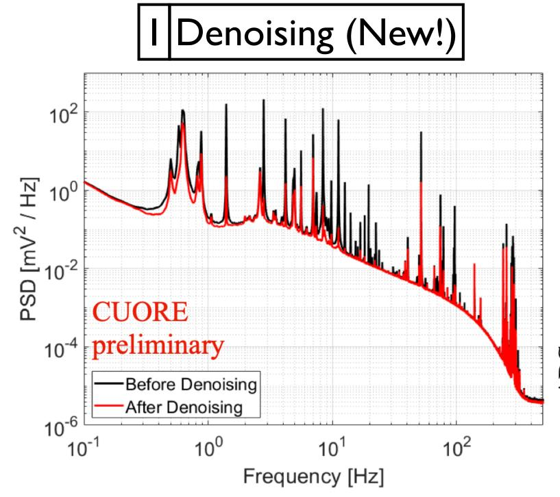
Noise is mitigated correlating vibrations with measurements obtained with auxiliary devices, i.e. microphones, antennae, accelerometers, seismometers
