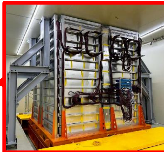
Plastic Scintillator Muon Detector (PSMD) (NIMA, 2022.167123)
