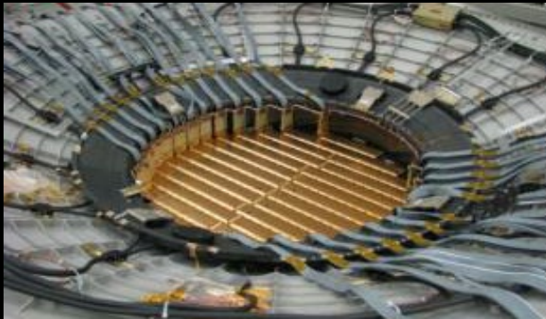
Ring Imaging Cerenkov (RICH) measure Z, E
