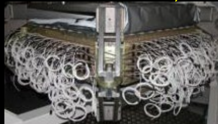
Electromagnetic Calorimeter (ECAL) measure E of e^+ , e^-
