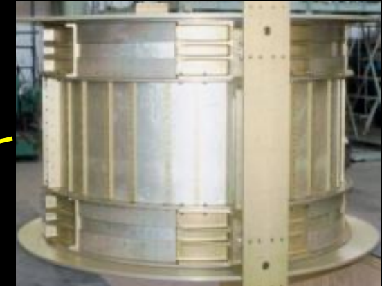
Anticoincidence Counters (ACC) reject particles from the side
