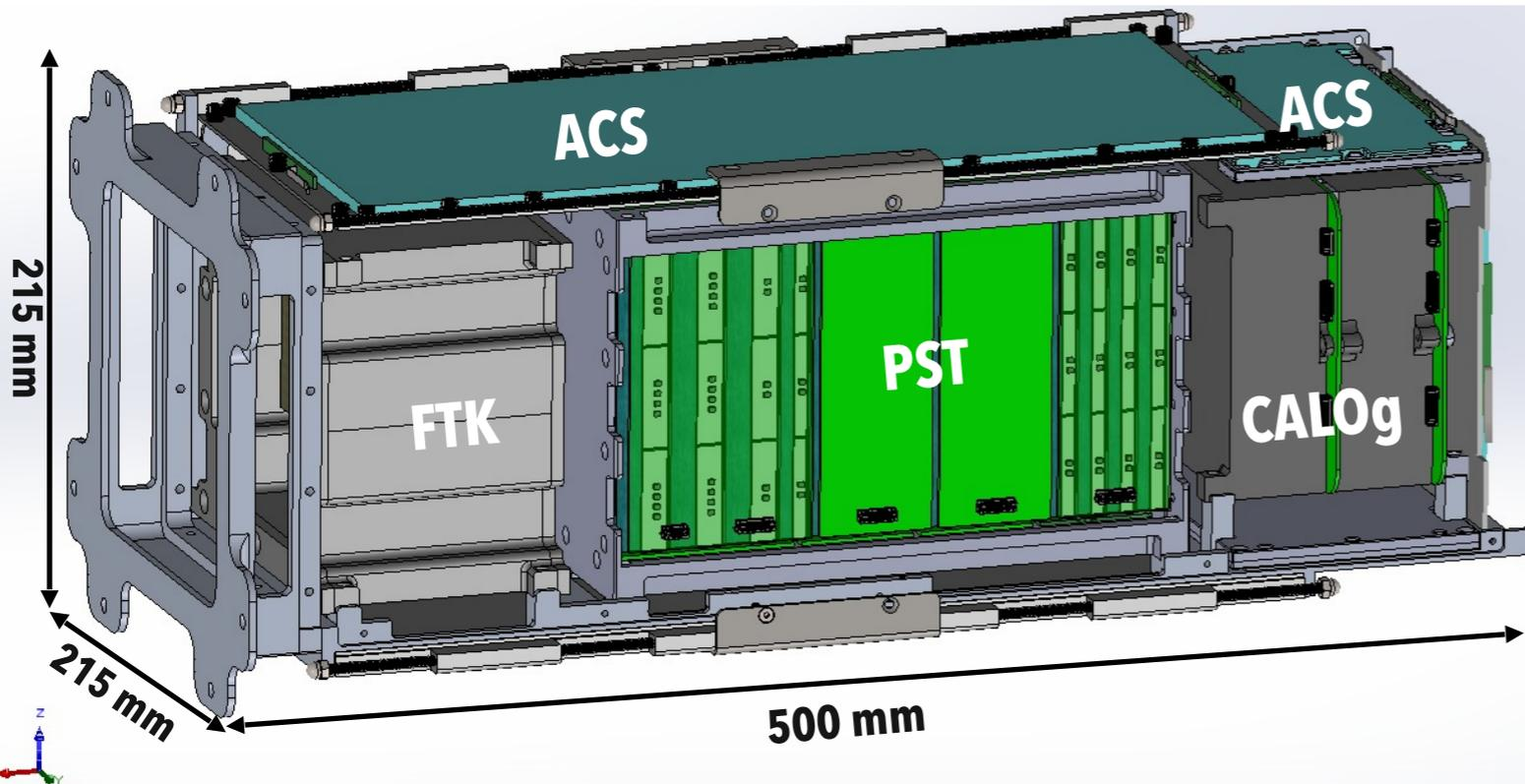
**ACS** (Anti-Coincidence System): a VETO for charged particle induced events made of plastic scintillator tiles and read out by SiPMs
