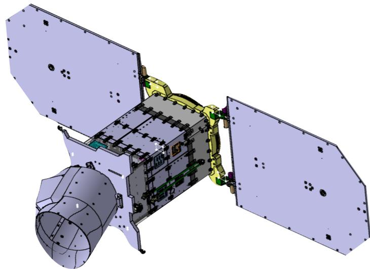
**NIMBUS (New Italian Micro BUS)**, the IRIDE SAR and Optical missions (Italian PNRR) platform is based on a new satellite bus concept which foresees a modular approach relying on standard trays.
