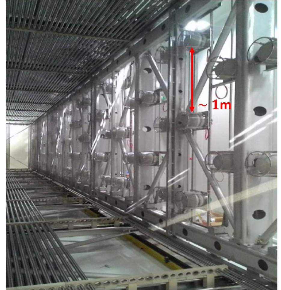
The new ICARUS PMTs mounted behind the wires of one TPC.
