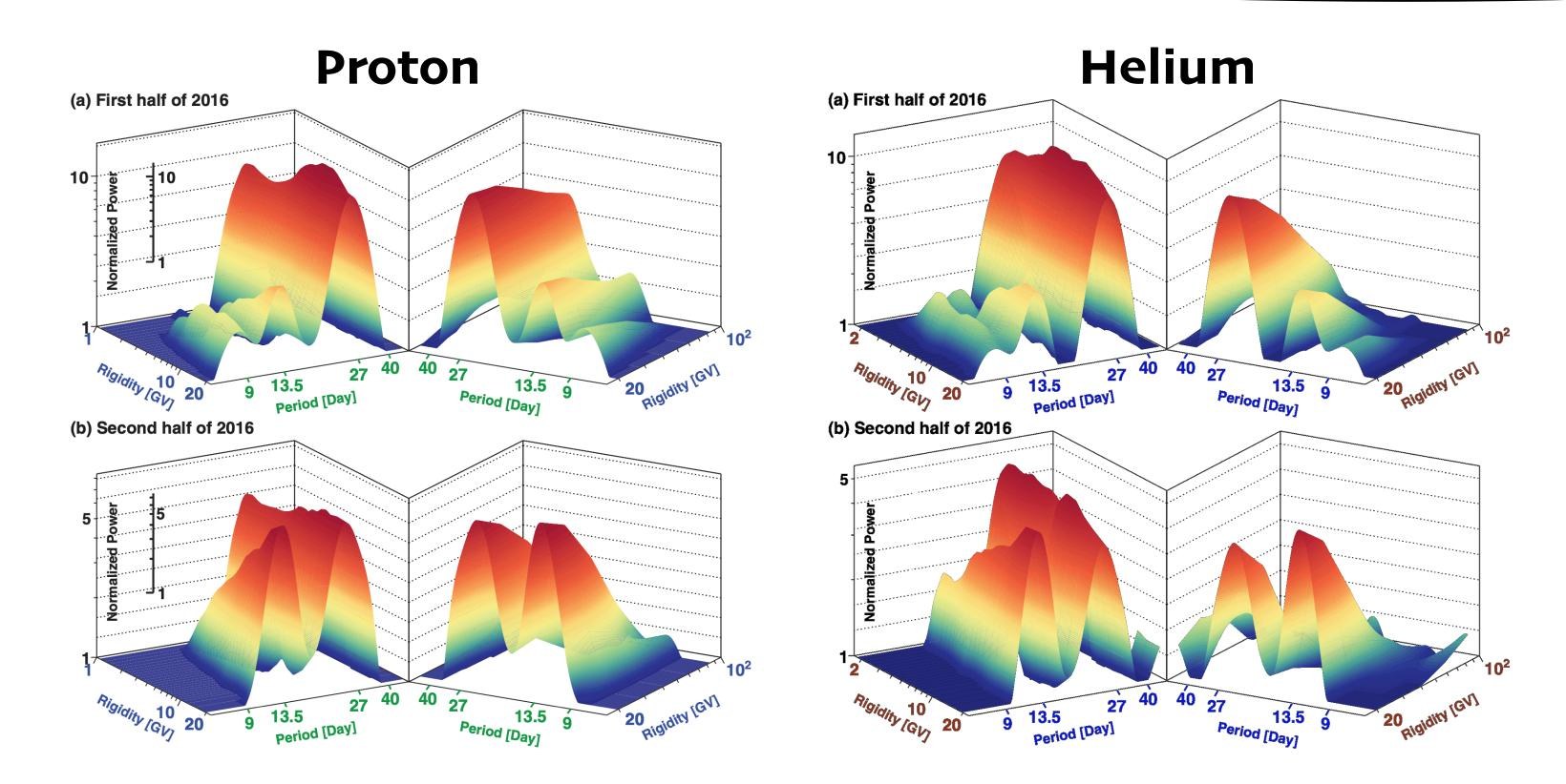
The above figures show the **rigidity dependence** of the intensity of periodicities for proton and helium fluxes. The **intensity** of 13.5 and 9 days periodicities, in both cases, reaches a **maximum** respectively at 10 GV and 20 GV. The AMS-02 result **is not compatible** with models that predict the **intensity of periodicities** to be constantly **decreasing** with increasing **rigidity**.
