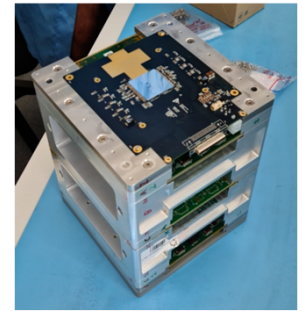
Figure 4 Assembly of MiniPAN. Timepix3 Quad is on the top. TOF scintillator has not been installed, yet.
