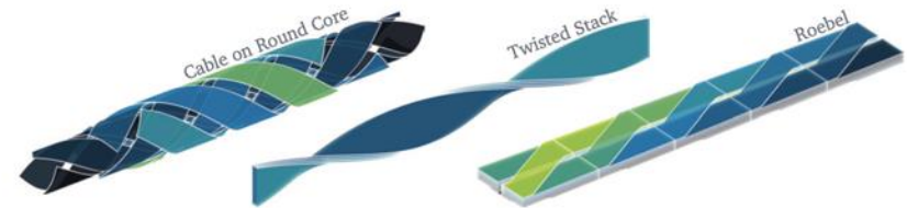
Figure 1.10. Three different geometries for assembling a cable with ReBCO coated conductor. Also refer to Table 1.2.
