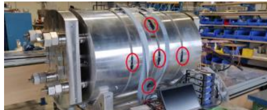
RMM1 flat-racetrack magnet during loading operation. The magnet achieved 16.4 T in the central cavity.
