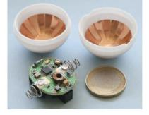
To allow these to be repaired it was necessary to find out exactly where they were without having to open the whole machine. The solution was to suck a ping-pong size ball fitted with a radio transmitter through the 3km magnet chain which extends from one LHC access point to the next.
