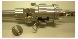
It was possible to follow the ball's progress using the LHC beam position monitoring system, which usually measures the beam position by picking up the radio signals generated by the beam. One such monitor is located every 54 m in the LHC.
