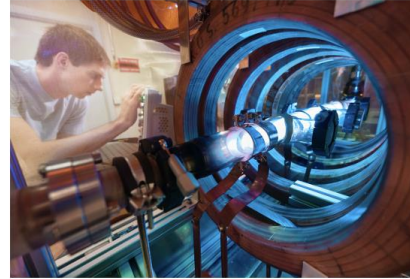
Plasma source 10m long, 4cm diameter, density 10^{14} - 10^{15} \text{cm}^{-3}
