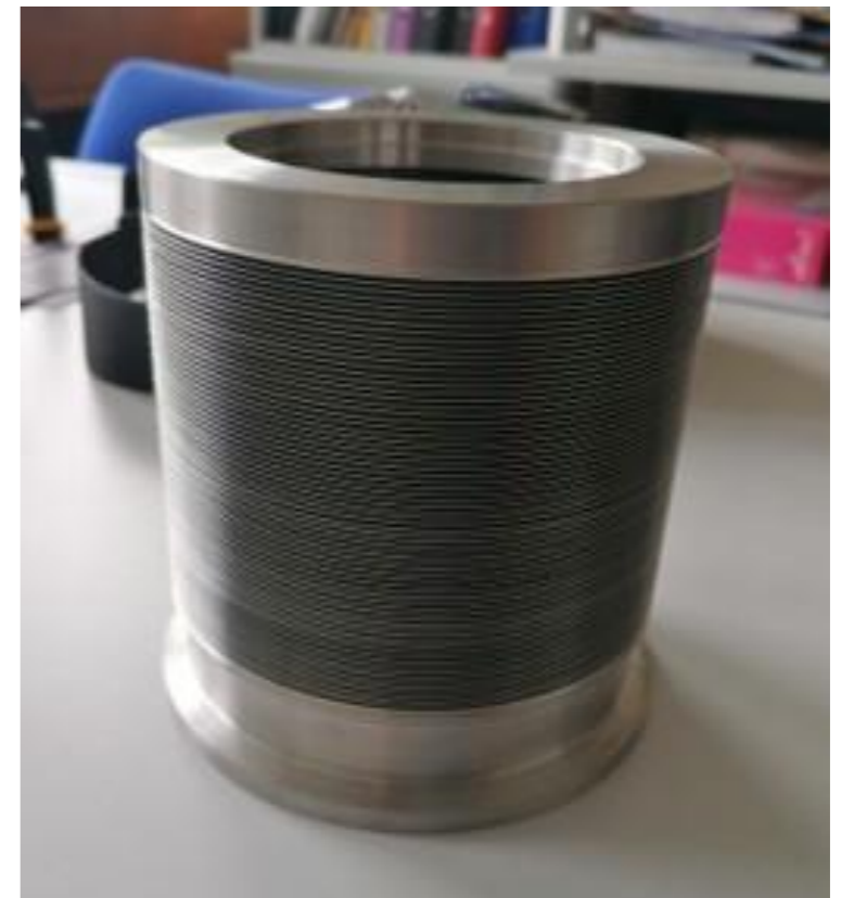
Spare bellow – tested to 20 bar
