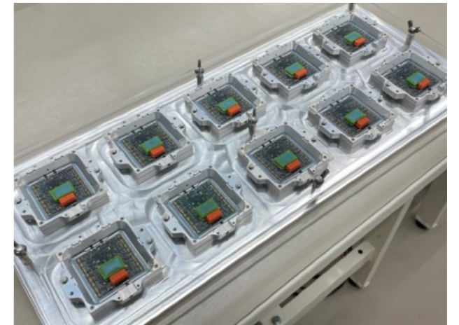
10 modules for parylene coating
