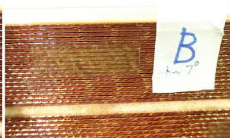
After repair of the damaged insulation
