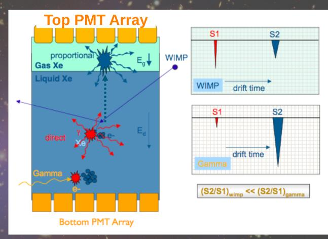
Single electron and single photon measurement sensitivity > 99.5% ER rejection via Ionization/Scintillation ratio (S2/S1)
