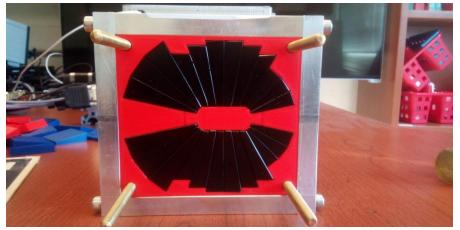
A prototype open midplane BF magnet was built and evaluated for mechanical integrity. Magnetic measurement confirmed a robust design with >1.5 Tesla in good field region, 10<sup>-3</sup> field accuracy. JLab radiation resilience tests in CEBAF began October 2023.
