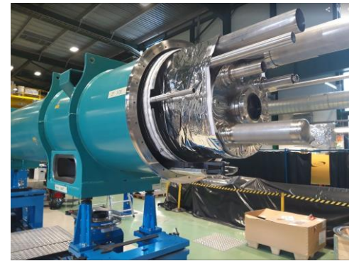
MBXFP1 in the cryostat
