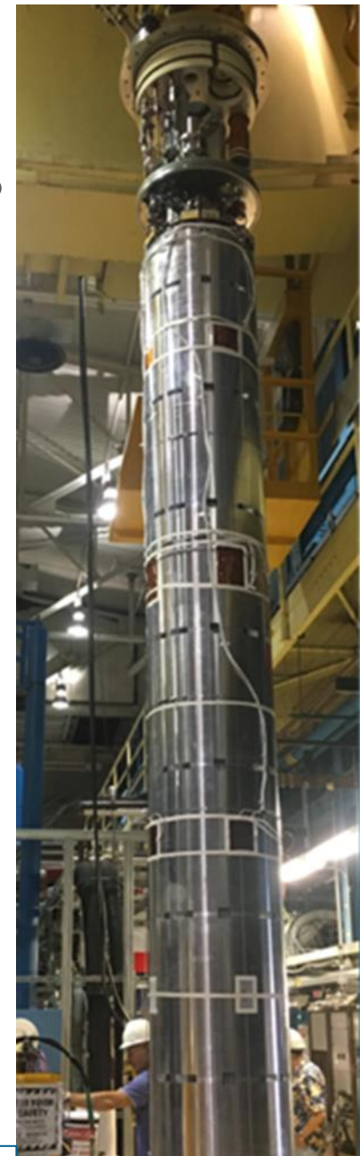
MQXFA magnet being moved to vertical test station at BNL 10
