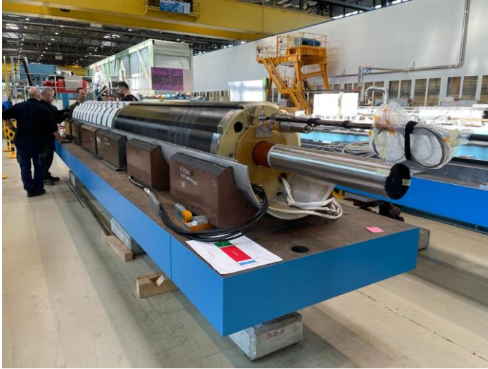
Assembly of long nested corrector into the cold mass
