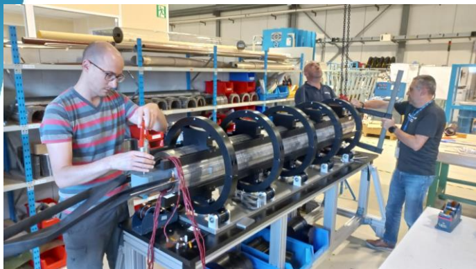
Assembly of inner collared dipole
