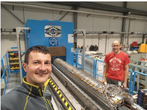
Inner dipole at collaring press
