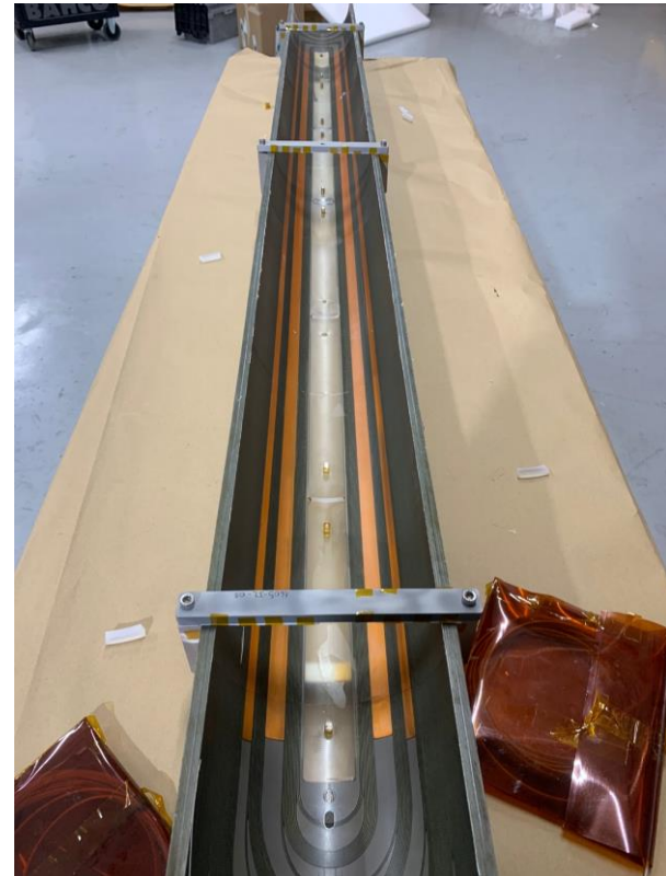
First long inner coil produced at Elytt 13 th HL-LHC Coll. Meeting – F. Toral - 25 th Sept 2023
