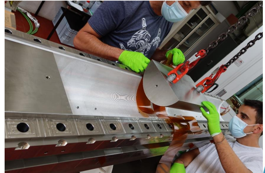
Impregnation mould assembly
