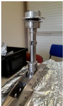
Components for cryostating Tuner frames & actuation
